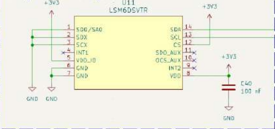
IMU (I2C ADDR: 0x6A)
